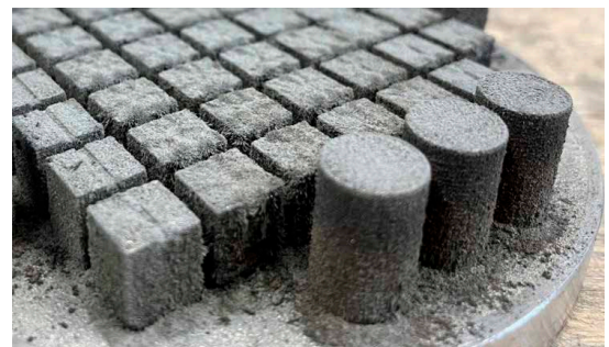
Figure 10: As-printed Nd-Fe-B samples which magnetically attract surrounding powder particles.
