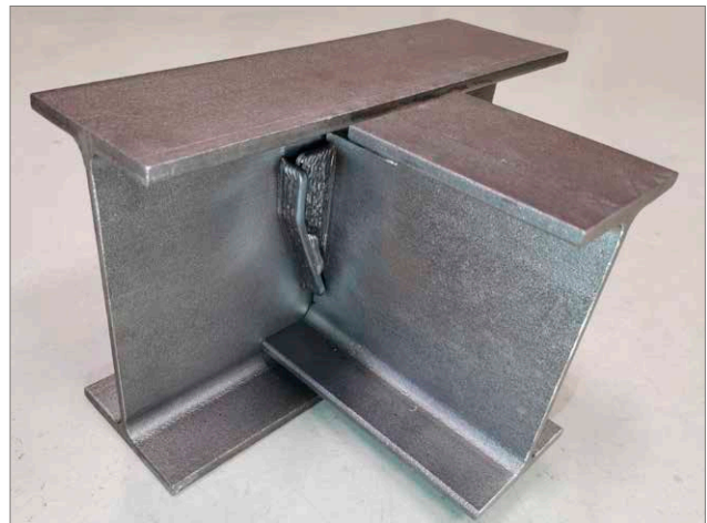
Figure 1: shear force connection for civil engineering application based on wire based additive manufacturing. Holzinger, Christoph: Additive Fabrication of Structural Steel Elements. PhD Thesis 2022, TU Graz, ITE picture: © Christoph Holzinger / TU Graz - ITE
