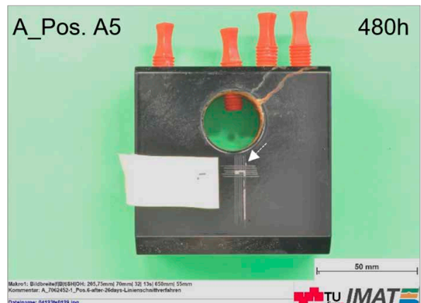
Cross-cut test (ISO 2409, s. arrow) of a polymer powder coating on a steel part - after 480 hours in salt spray chamber (ISO 9227).
