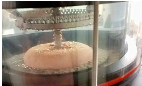
IEHCC test of a zinc-coated timber screw in salt-solution / counter electrode above
