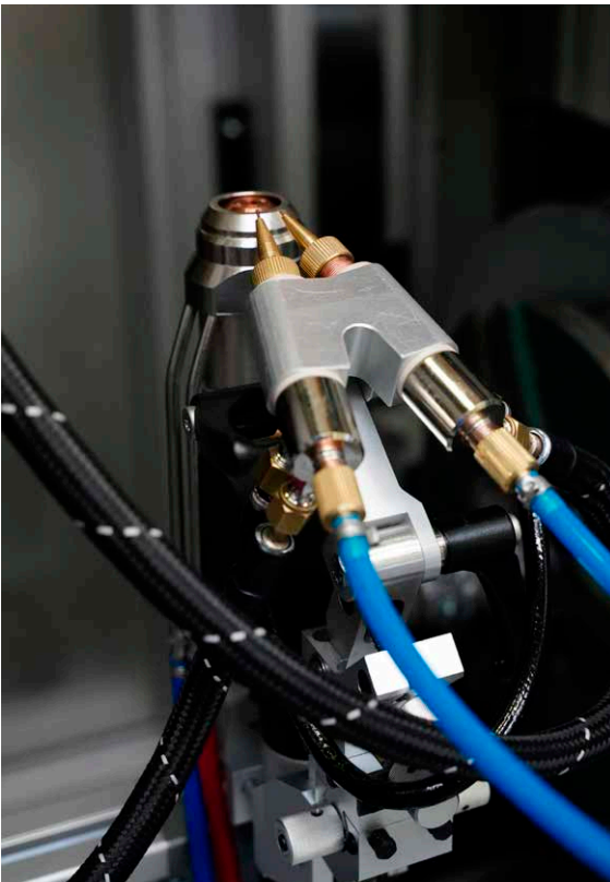
Torch in overhead position with two wire feeds
