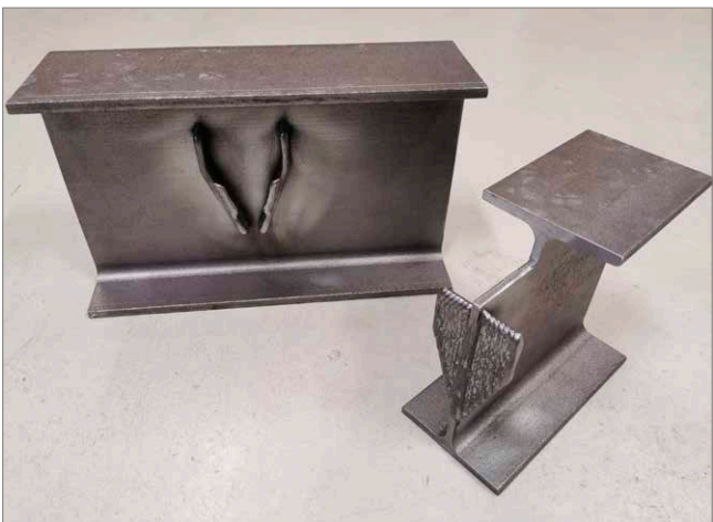
Figure 1: shear force connection for civil engineering application based on wire based additive manufacturing. Holzinger, Christoph: Additive Fabrication of Structural Steel Elements. PhD Thesis 2022, TU Graz, ITE picture: © Christoph Holzinger / TU Graz - ITE
