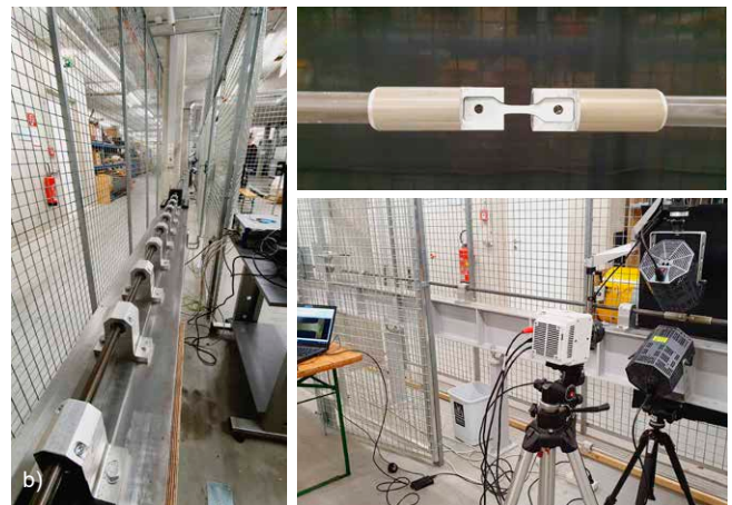
Figure 5: Universal Split Hopkinson Testing Machine [VSI] – tensile tests at RT/100°C and up to strain rates of 1000 [1/s]
