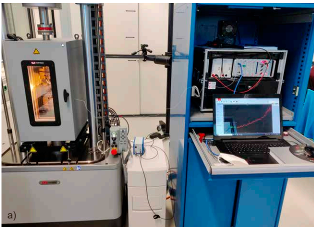
Figure 4: Intron ELECTROPULS® E10000 – tensile tests up to 300°C and strain rates from 0.001 to 1 [1/s]
