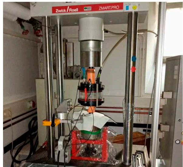
Installed IEHCC at the PSA hydraulic tensile test machine
