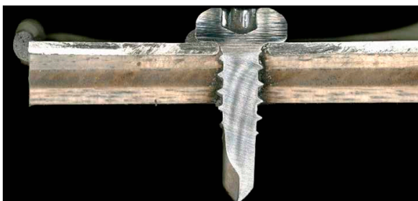
Figure 8: Cross-section of an adhesive and screw-bonded aluminum-wood component.
