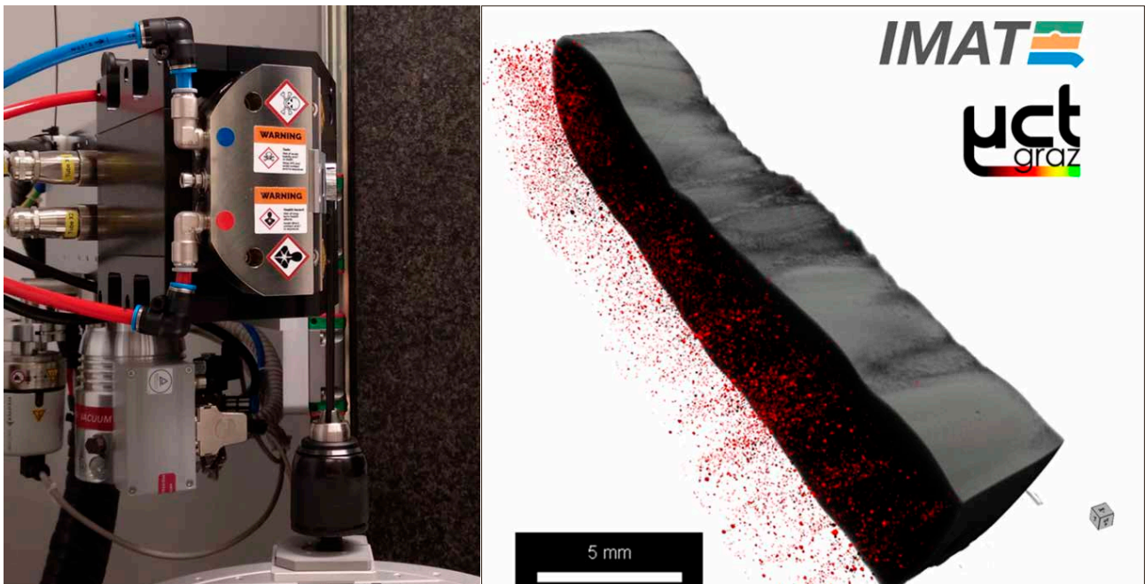
Figure. \mu CT measurement carried out with Tescan UniTOM XL. Pore distribution of a wire arc additive manufactured aluminium alloy (We3D project). Left: Setup of the measurement. Right: Spatial distribution of pores within the sample.
